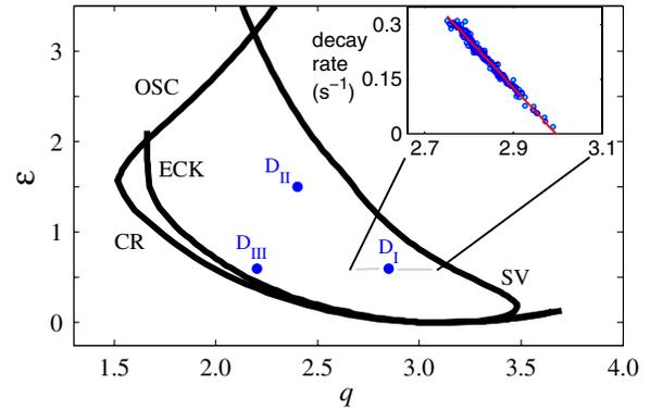
FIG. 2 (color online). Stability balloon at  $\text{Pr} = 0.84$  showing various instabilities (CR, cross roll; ECK, Eckhaus; SV, skew varicose; OSC, oscillatory) of the straight roll state along with the parameters at which the experimental data were taken for the three data sets.  $D_I = (0.60, 2.85)$ ,  $D_{II} = (1.50, 2.40)$ , and  $D_{III} = (0.60, 2.20)$ . The inset plot shows the disturbance decay rate ( $\text{s}^{-1}$ ) as a function of wave number  $q$  at fixed  $\epsilon = 0.60$ .
