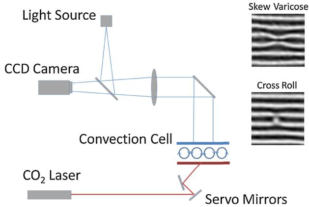
FIG. 1 (color online). Experimental setup includes a shadowgraph visualization as well as a system for optical actuation. Insets are observed responses to local perturbations at different parameter values. These disturbances represent the local version of the skew-varicose and cross-roll instabilities, respectively, of the unbounded system.
