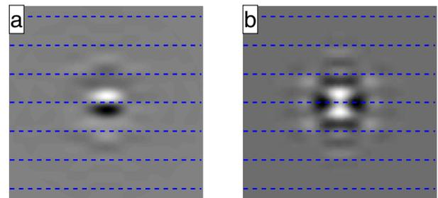
FIG. 3 (color online). (a) The fundamental dominant and (b) subdominant mode extracted at  $D_1$ . Dashed lines mark the approximate locations of the hot fluid of the underlying base state; cold fluid lies between the dashed lines.
