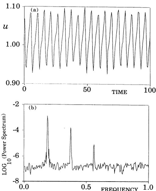
FIG. 4. (a) Time series and (b) power spectrum of the streamwise velocity  $u$  measured by laser Doppler velocimetry at  $x = 3.9$  downstream of cylinder 18,  $y = 0$ , and  $z = -5.2$  for  $R = 170$  and  $k_i = 0.42$ .
