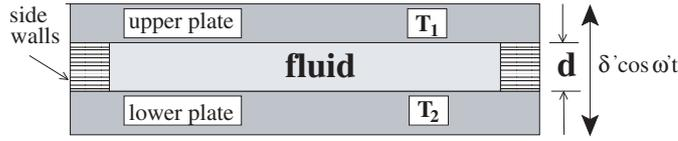
**Figure 1.** Fluid motion in the layer of depth  $d$  is driven both by the imposed temperature difference  $\Delta T = T_2 - T_1$  and the vertical oscillations  $\delta' \cos \omega t$ . In addition to the Rayleigh–Bénard convection parameters of  $Pr$  and  $R$ , this system is characterized by two nondimensional modulation parameters  $\delta Fr$  and  $\omega$  (see text).
